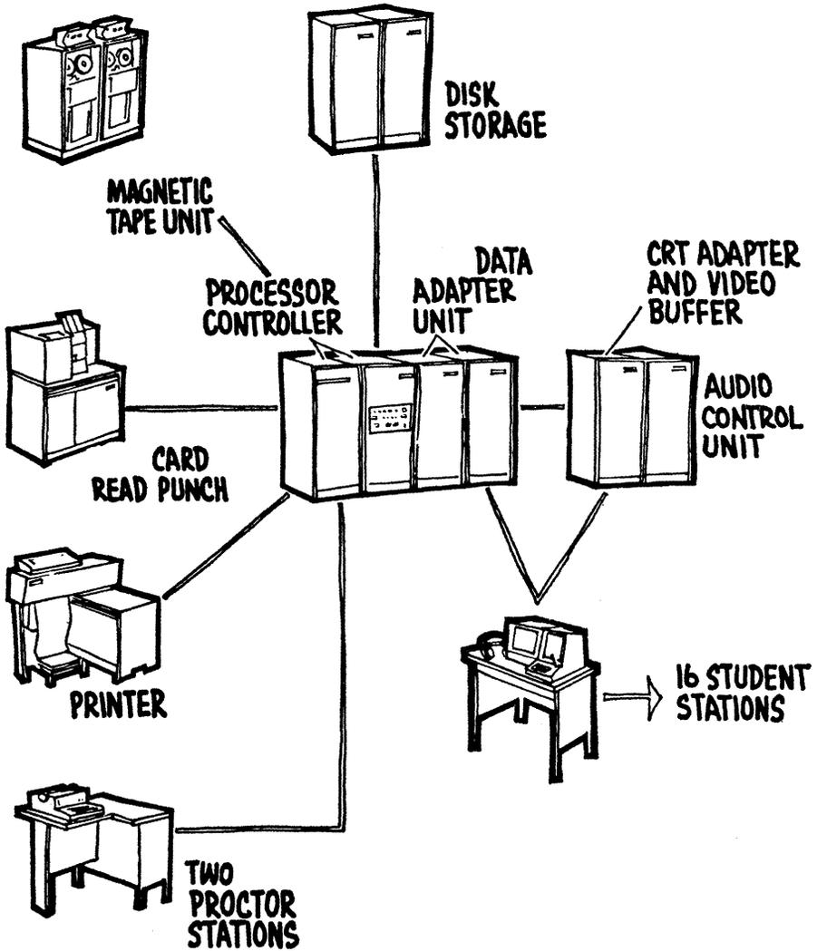
FIG. 1. System configuration for computer-assisted instruction.
